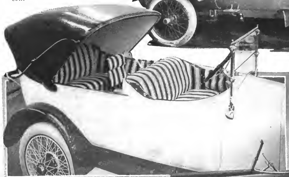
The Cunningham boat-shape body on the new eight-cylinder chassis. Note that the sides of the body are rounded inward at the upper edges so as to bend smoothly into the center cowl
